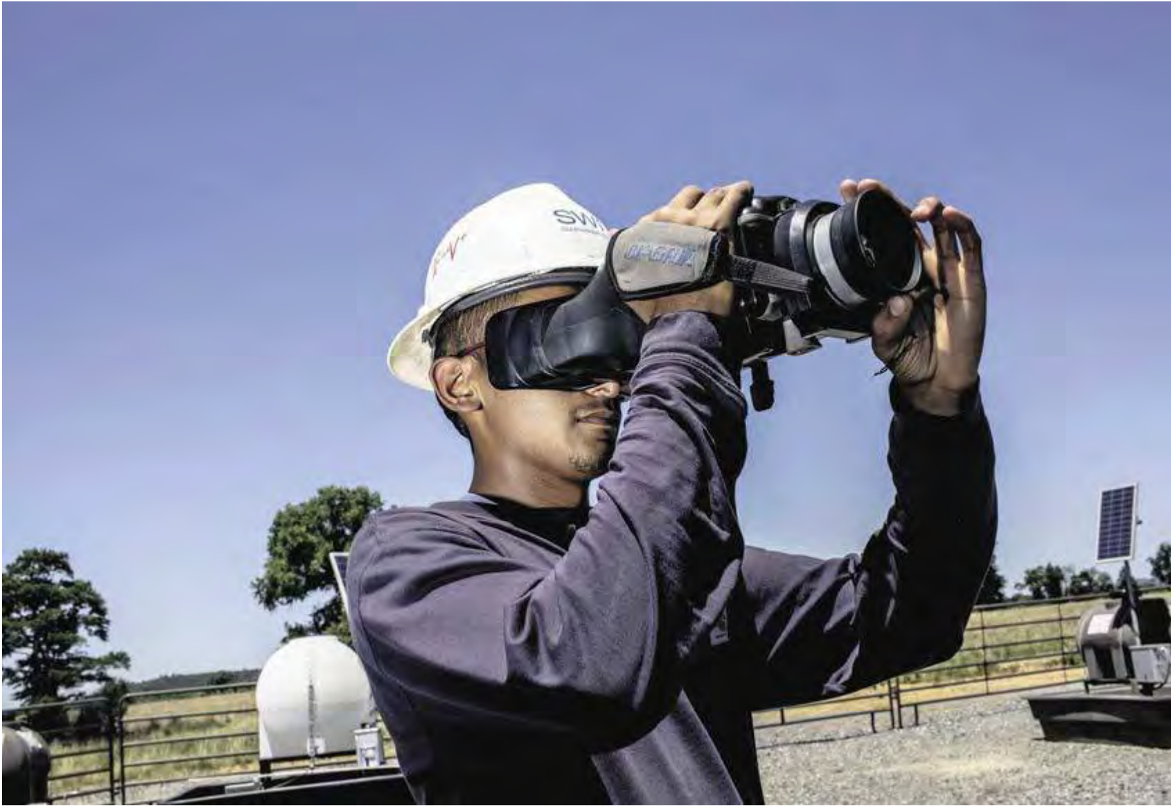
Ronal Torres, a technician for Southwestern Energy, using an infrared camera to search for methane leaks in Damascus, Ark. Methane is a more potent greenhouse gas than carbon dioxide.
