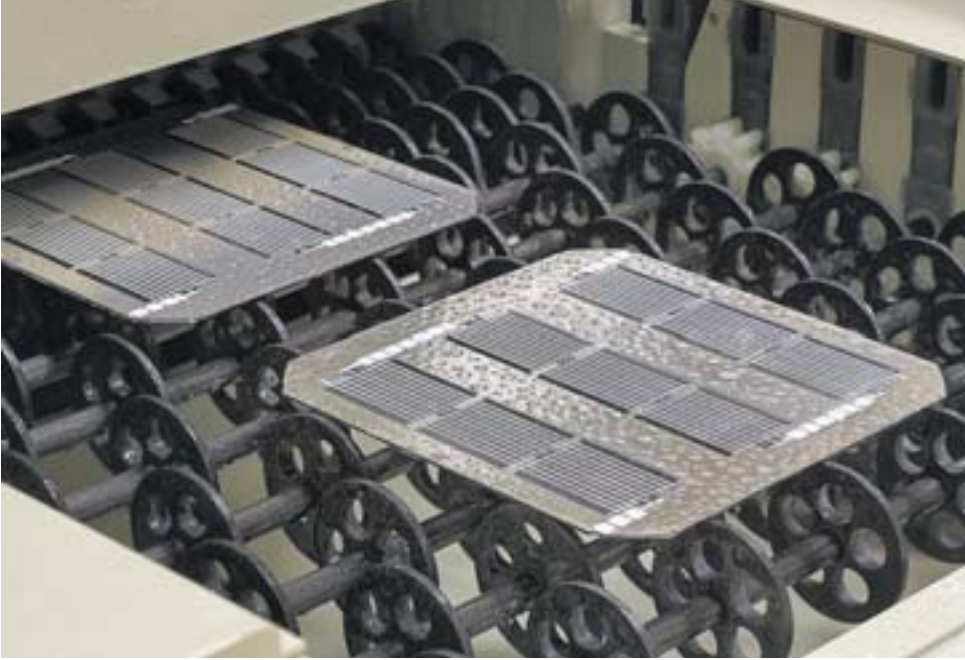
Silicon wafers are processed to make high-capacity batteries at Enovix’s pilot unit in Fremont, Calif.
