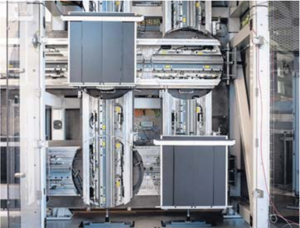
A view of a prototype elevator that can move vertically or horizontally at a Spanish test facility.
